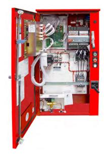
**Description** – Firetrol® FTA1000 Full Voltage Fire Pump Controllers are intended for use with electric motor driven fire pumps where the capacity of the power source permits full voltage starting. Full voltage is applied to the motor as soon as the controller is actuated. The controller monitors, displays and records fire pump system information.
